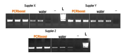
**Figure 4:** 10ng gDNA were amplified using human  $\beta$ -actin primers in PCRboost<sup>TM</sup> or water using Taq DNA polymerases from 3 different suppliers (X,Y,Z). -: no Taq control. L: ladder
